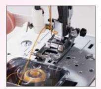
Simply lower the lever and turn it back and forth. This single action makes it easy to thread the needle.
